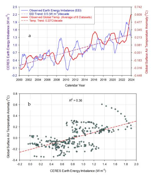
**Figure 13.** Relationship between Earth's Energy Imbalance (EEI) measured by CERES and GSAT anomalies based on 6 global datasets: (a) Comparison of GSAT and EEI time series representing 13-month running means; (b) Linear correlation between EEI and GSAT. The dashed red line is a linear regression. EEI only explains 36% of the GSAT interannual variability, while the solar forcing explains 83% of it (Figure 9).
