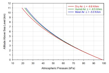
**Figure 16.** Atmospheric pressure as a function of altitude according to the barometric formula (Equation (18c)) for three different lapse rates: dry adiabatic (L = -0.0098 K/m), humid environmental (L = -0.0065 K/m), and moist adiabatic (L = -0.005 K/m). Note that variations of the lapse rate only have a minor impact on the decrease of pressure with altitude.
