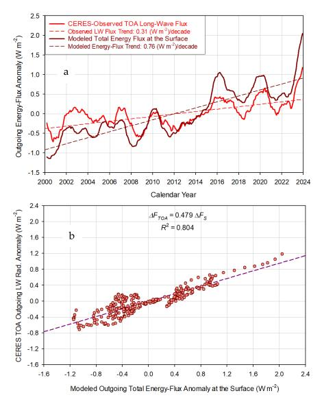
**Figure 14.** Observed outgoing LW flux at the TOA by CERES and modeled total energy flux at the surface by Equation (17) using the GSAT record in Figure 5b as input: (a) Time series and trends of the observed and modeled fluxes; (b) Relationship between the modeled surface total energy-flux anomalies and the observed TOA upwelling thermal-flux anomalies. The dashed magenta line is a linear regression. The magnitude of the TOA flux anomalies is, on average, 47.9% the size of surface fluxes.
