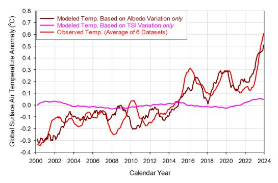
**Figure 11.** Global surface temperature changes predicted in response to observed variations of TOA TSI (Equation (8)) and the planetary albedo (Equation (15a)) over the CERES monitoring period. These are compared to measured GSAT anomalies. The observed multi-decadal warming trend and the El Niño-Southern Oscillation (ENSO) cycles are almost entirely explained by changes in the Earth's albedo, while TSI only has a small, almost inconsequential contribution.
