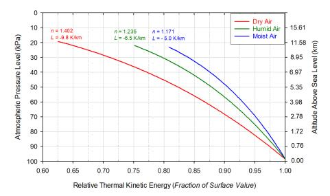
**Figure 17.** Decrease of the thermal kinetic energy in the troposphere *relative* to the thermal kinetic energy of air at the surface for a standard atmosphere under 3 scenarios defined by different polytropic indices and temperature lapse rates applicable to dry, humid, or moist environments, respectively. According to the Gas Law, the thermal kinetic energy of air is defined by the product *PV*.
