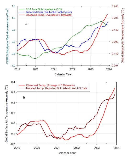
**Figure 10.** Illustrating the cause of the 2023 global heat anomaly: (**a**) Observed GSAT in relation to changes of TSI and the absorbed shortwave radiation measured by CERES; (**b**) Observed GSAT in relation to the modeled global temperature response to solar forcing (TSI and albedo combined) according to Equation (16). The observed GSAT lags the modeled GSAT because global temperature lags changes in the absorbed solar flux.
