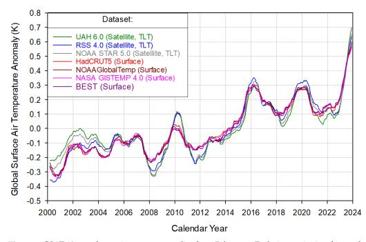
**Figure 3.** GSAT 13-month running mean anomalies from 7 datasets. Each time series is referenced to its respective mean over the period March 2000–December 2023. The satellite-based datasets report temperature changes in the lower troposphere (TLT) measured by Microwave Sounding Units (MSU), while surface-based databases are derived from thermometer readings on the ground.
